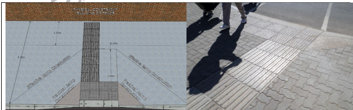
Figure 5: Effective and practical ramp construction.
